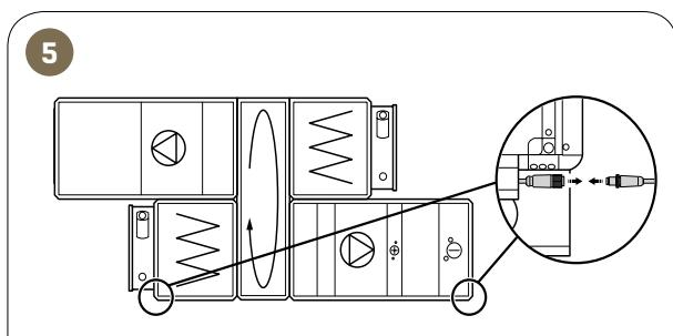
**UK** - Outdoor temperature sensor (fasade sensor). (Connection see wiring diagram)
