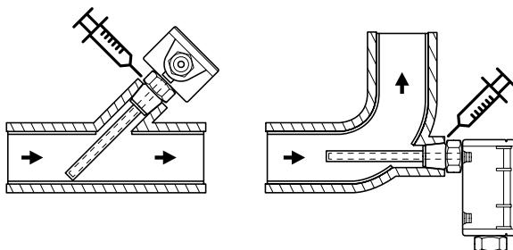
**UK** - Duct pressure transducer **SE** - Kanaltryckgivare **FI** - Kanavapaineanturi
