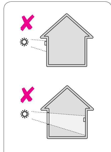
**UK** - Room mounted CO<sub>2</sub> transducer (Connection, see wiring diagram)
